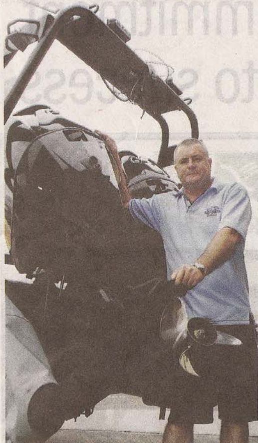
Big horses: Steve Britton with a partially built rapid-intervention boat, powered by twin 500-horsepower outboards, destined for the Northern Territory Police.
